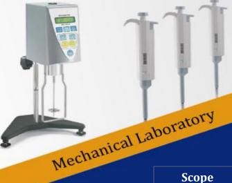
Piston pipette :  $10 \mu l$  to  $1000 \mu l$
